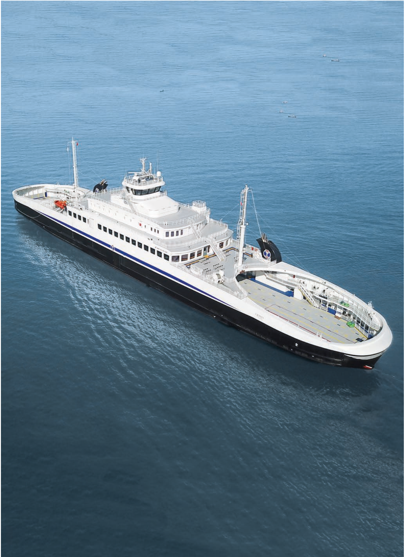
LNG-Powered RoPax Ferry Færøy 2 x SRE 560 CP (2700 kW each)
