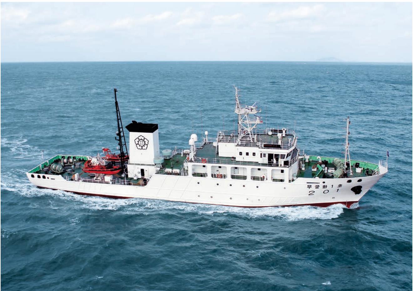
Fishery Supervision Vessel Mugunghwa 2 x SCP 654 (1750 kW each)
