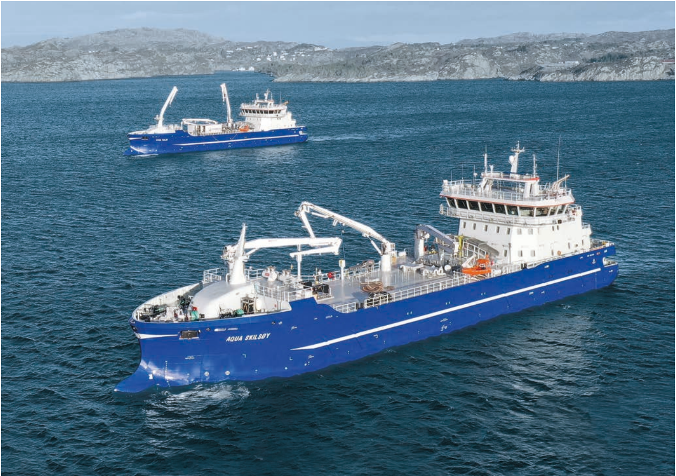
Live Fish Carriers Aqua Maløy, Aqua Skilsøy 2 x SRP 360 (1400 kW each), 2 x STT 1 CP (400 kW each)
