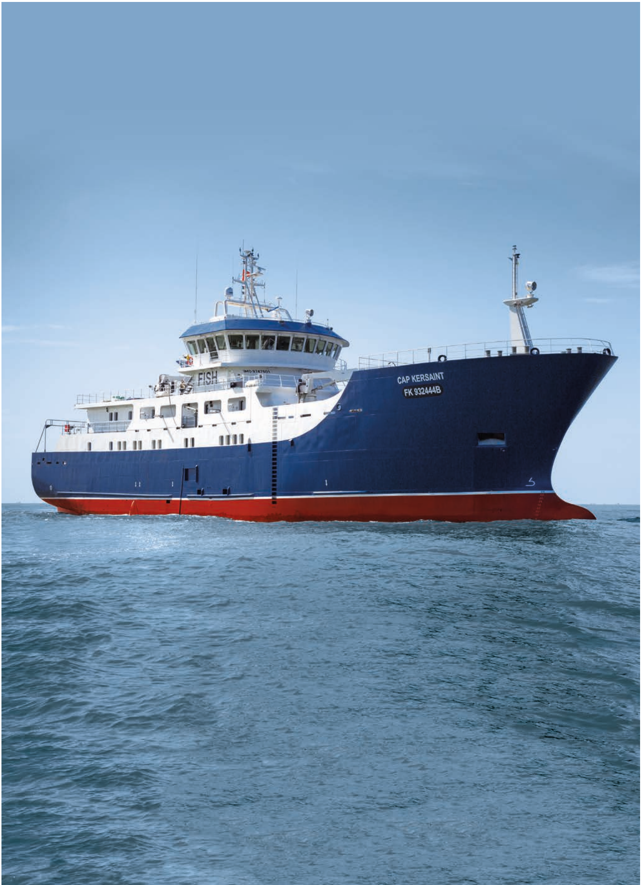
Longliner Cap Kersaint 2 x STP 340 (1000kW each)
