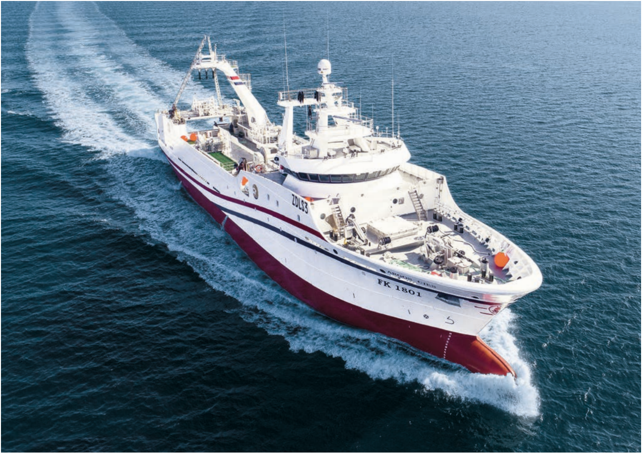
Trawler Argos Cies 1 x SCP 1004 (3000 kW), 1 x STT 1 (400 kW)
