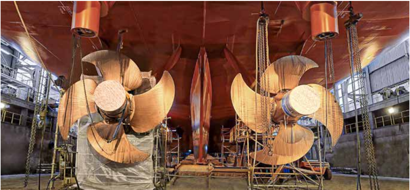
Under construction: two SCHOTTEL ControllablePropellers type SCP 1294 with 9,600 kW each for the ro-ro ferry Tendor Ocean at the Flensburger Schiffbau-Gesellschaft (FSG) shipbuilding company
